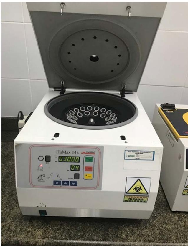
Fig 2: HuMax centrifuge where tubes are placed.
